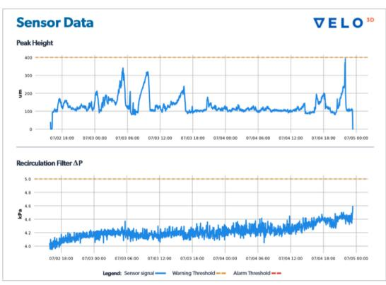
Taken directly out of the Assure build report and showing actual data from the Sierra Turbines project, see data related to Peak Height and Filter Recirculation. Peak Height measures concerns against protrusions, and the Recirculation Filter measures the life of the filter during the build. Both show no concern as the sensor readings are under the warning threshold.
